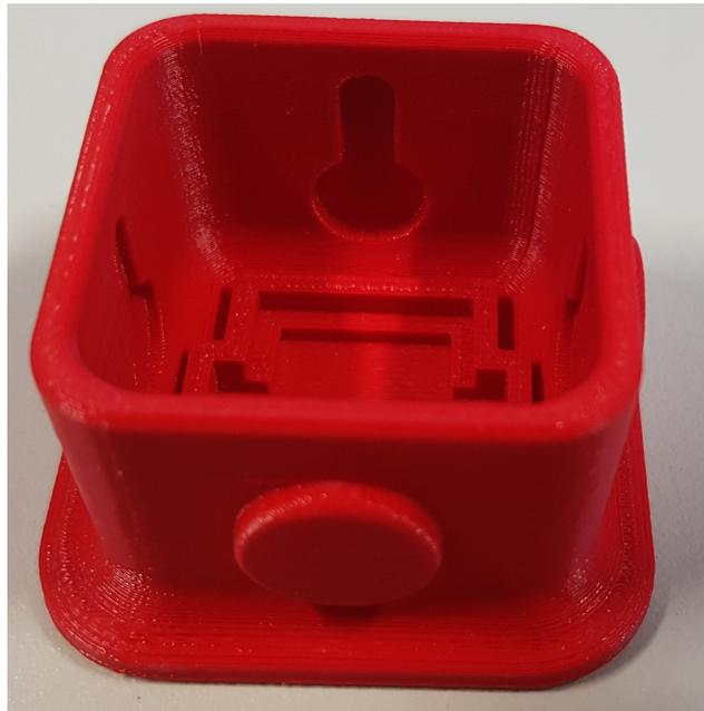
Figure 3.11: *Redesign of the transmission mass body.*
