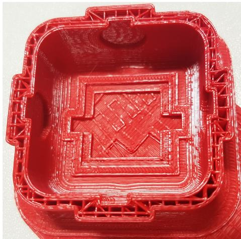
Figure 3.7: *Image of a partially completed print showing the inner lattice between the faces of the shape.*
